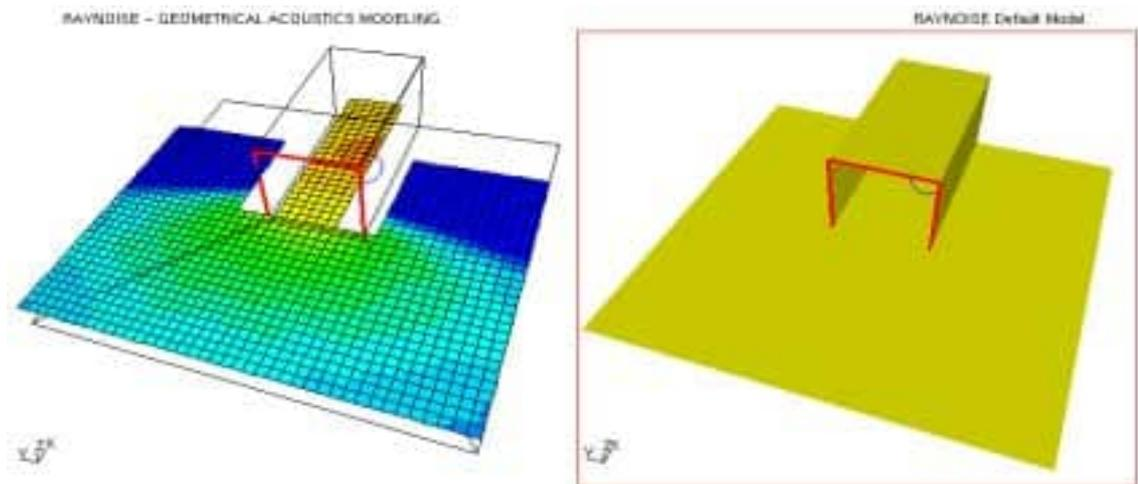
Figure 3.3–5 Diffracted field at tunnel exit
