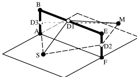
Figure 3.3-3 Three diffraction paths around a screen
