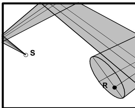
Figure 3.1-6 Cone propagation through physical boundaries
