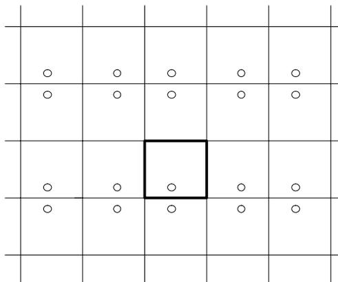
Figure 3.1–3 Constructing Mirror Image Sources
