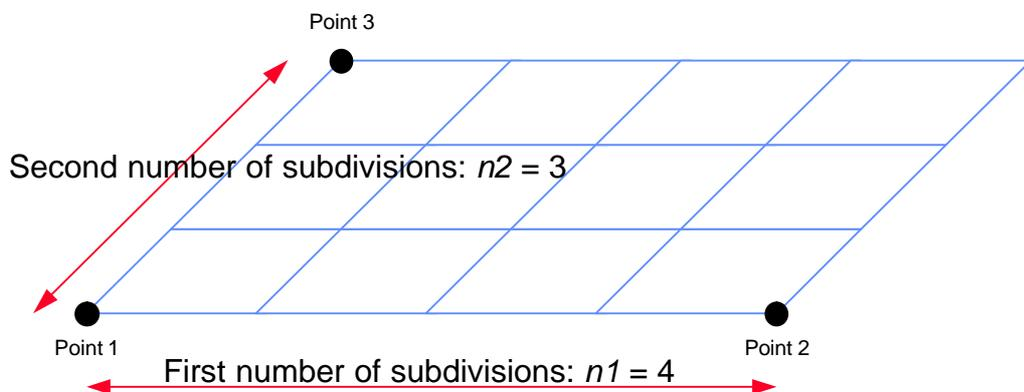
Figure 7.4–3 Geometry of an area source
