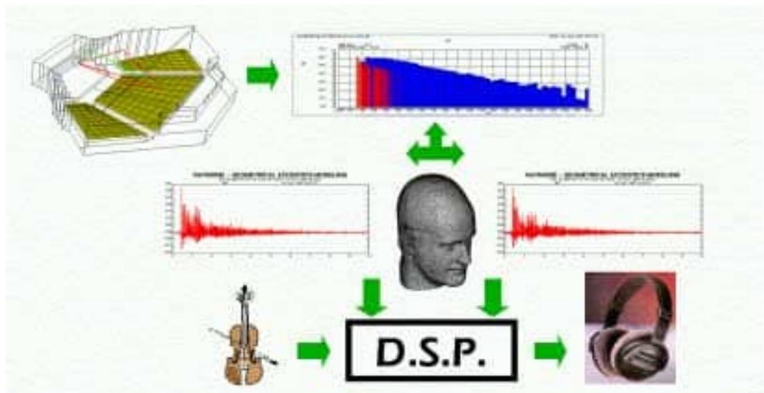
Figure 3.7–1 Flow diagram of the auralization process
