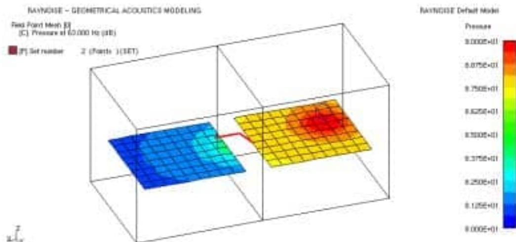
Figure 3.6–2 Example of sound transmission between rooms
