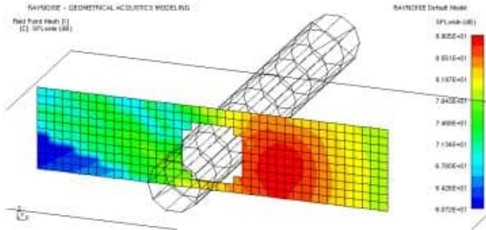
Figure 3.3–9 Sound field in dB–lin around a cylinder, with floor
