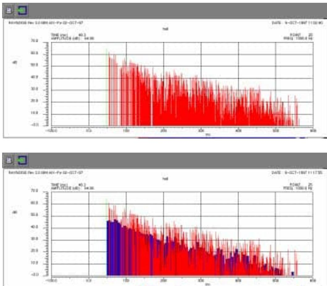
Figure 3.5–1 Echogram (a) without (b) with diffuse reflections
