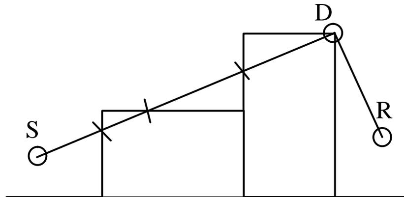
Figure 3.3–6 Multiple edge diffraction, approximated by an equivalent first-order diffraction.
