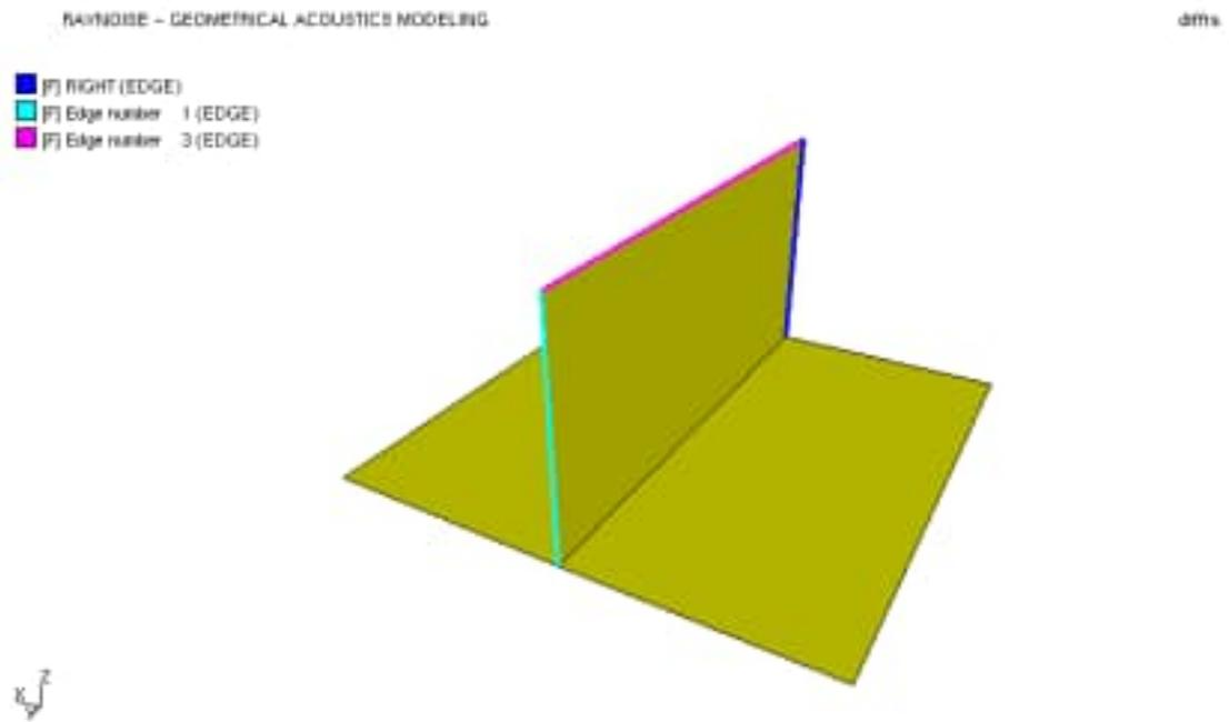
Figure 6.4-2 Free edges which may be picked as diffraction edges
