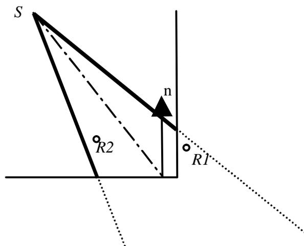
Figure 3.1-13 Receiver R1 gets an erroneous contribution, Receiver R2 gets a correct contribution
