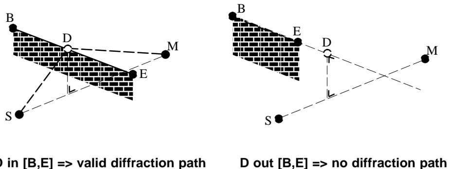
Figure 3.3–1 *S(image) source, M receiver, BE diff edge, D diff point*
