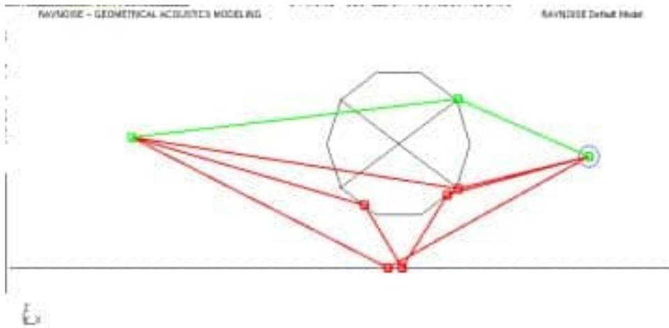
Figure 3.3–10 Ray paths from source to receiver, including reflections and diffractions.
