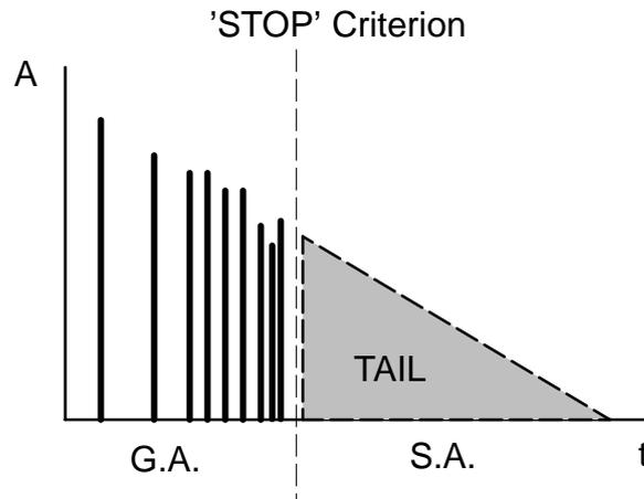
Figure 3.1–15 Transition from Geometrical Acoustics to Statistical Acoustics
