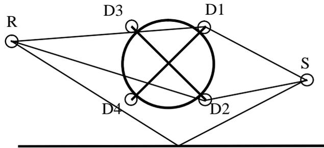
Figure 3.3–7 Diffraction paths around a cylindrical object
