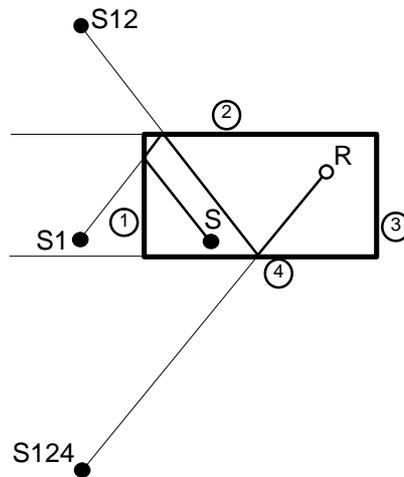
Figure 3.1–2 Third–order mirror image and corresponding reflection path
