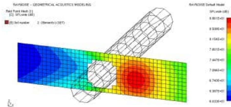
Figure 3.3–8 Sound field in dB–lin around a cylinder, no floor
