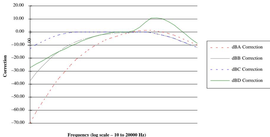
Figure 10.3–4 A, B, C and D dB–filters (corrections in dB).
