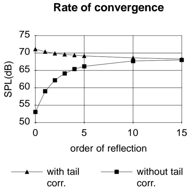
Figure 3.1–16 Faster convergence with tail correction
