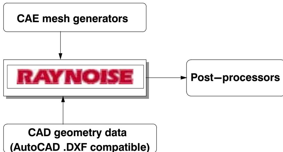
Figure 5.3–1 Data exchange with pre-/post-processors and CAD
